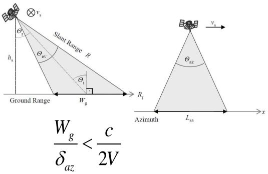
Swath-to-azimuth resolution constraint for a monostatic platform system...
