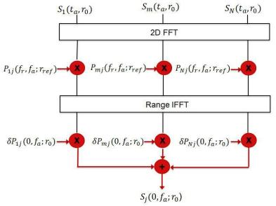
The coherent combination of the multiple receiving signals allows to reduce the PRF of transmitting signal by a factor of N (where N is the number of receivers), hence enabling to enlarge the width of the non-ambiguous swath on the ground, without arising of azimuth ambiguities
