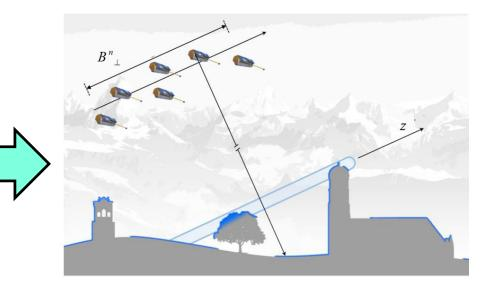
Multi-Baseline Single-Pass interferometry allows to drastically improve the DEM (Digital Elevation Model) accuracy
