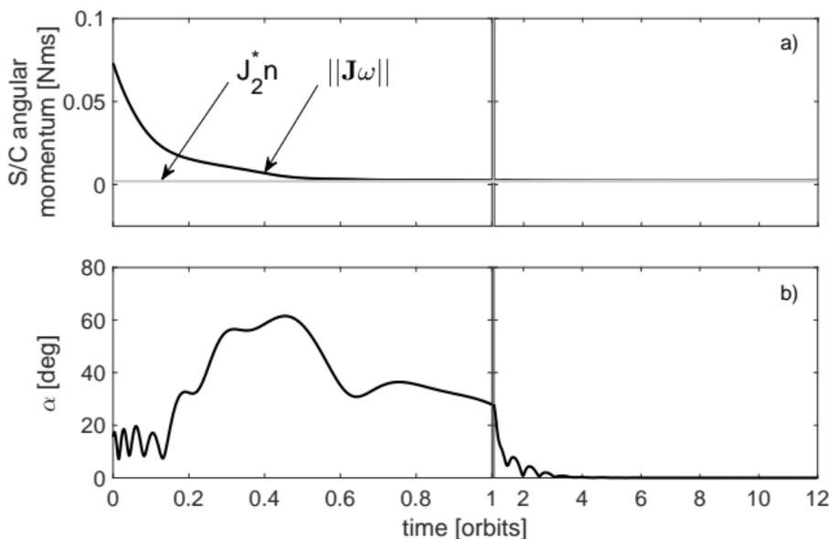
$\alpha = \cos^{-1}(\hat{\sigma} \cdot \hat{e}_2)$  is the angular distance between the desired spin axis  $\hat{e}_2$  and the target direction  $\hat{\sigma}$
