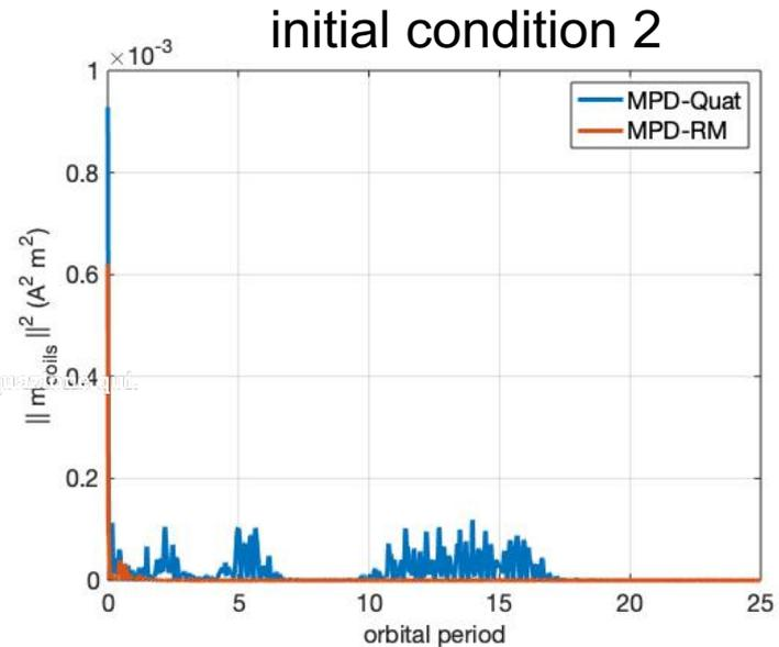
“energy” consumption  $\approx \int_0^{t_{fin}} \|\mathbf{m}_{coils}(t)\|^2 dt$
