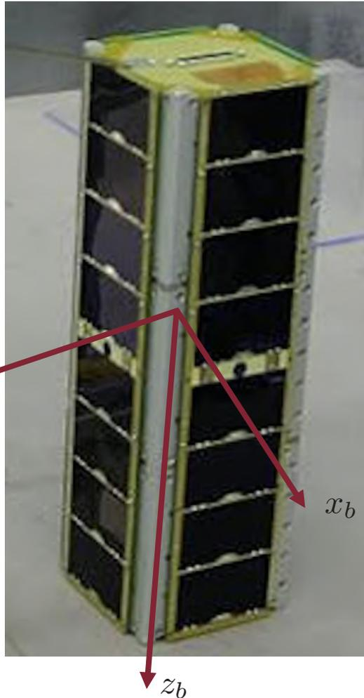
$$J_x = J_y = 4.09 \cdot 10^{-2} \text{ kg m}^2 \quad J_z = 6.5 \cdot 10^{-3} \text{ kg m}^2$$
