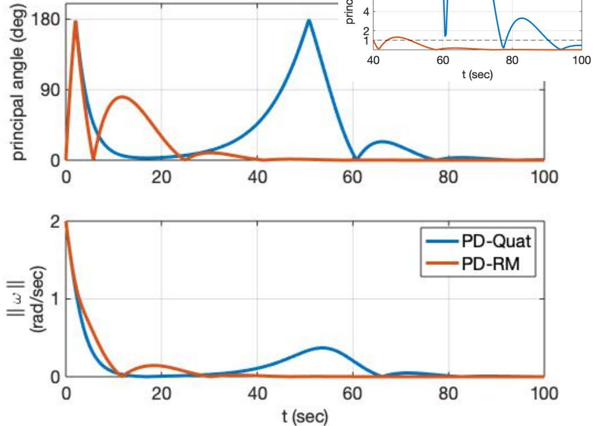
$$\text{settling time} = \begin{cases} 90.4 \text{ sec} & \text{PD - Quat} \\ 50.8 \text{ sec} & \text{PD - RM} \quad (-44\%) \end{cases}$$
