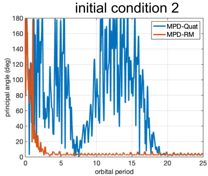
$$\text{Integral Time Absolute Error (ITAE)} = \int_0^{t_{fin}} t \text{ principal angle}(t) dt$$
