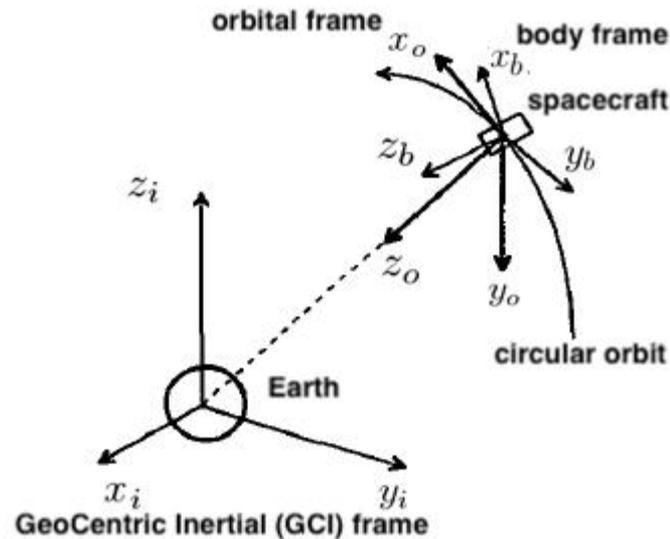
**objective:** stabilize attitude so that body frame is aligned with orbital frame (camera pointing to Earth)
