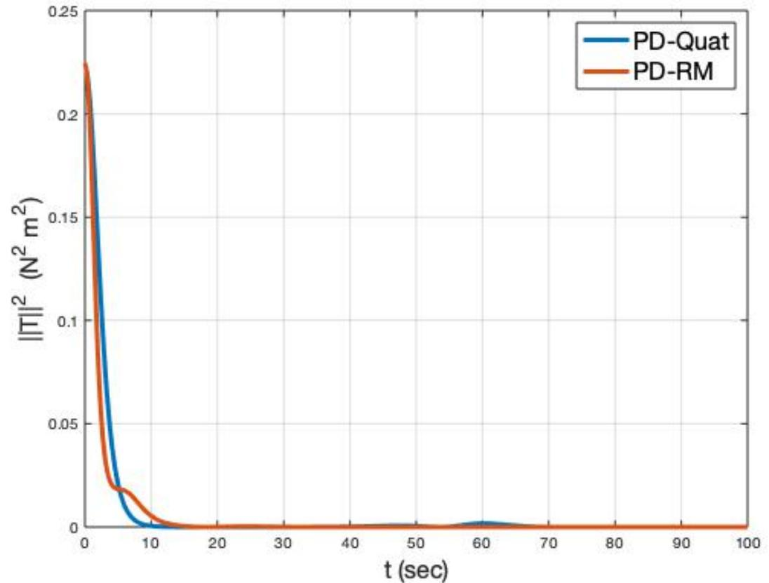
$$\text{energy consumption} \approx \int_0^{t_{fin}} \|\mathbf{T}(t)\|^2 dt = \begin{cases} 0.62 \text{ N}^2 \text{ m}^2 \text{ sec} & \text{PD - Quat} \\ 0.51 \text{ N}^2 \text{ m}^2 \text{ sec} & \text{PD - RM} \quad (-18\%) \end{cases}$$
