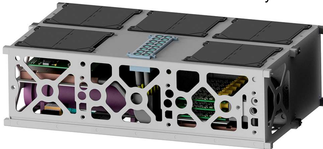
MLHS instrument configuration for 6U CubeSat
