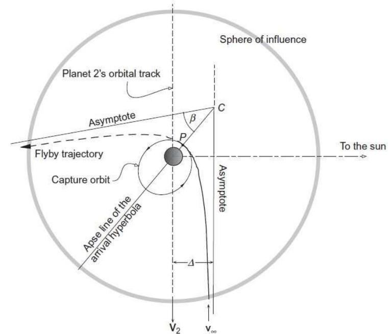
Figure 5. Spacecraft approach trajectory for a Hohmann transfer to an outer planet from an inner one. P is the periapsis of the approach hyperbola.
