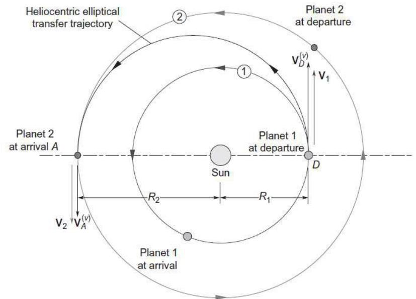
Figure 2. Departure of a spacecraft on a mission from an inner planet to an outer planet.
