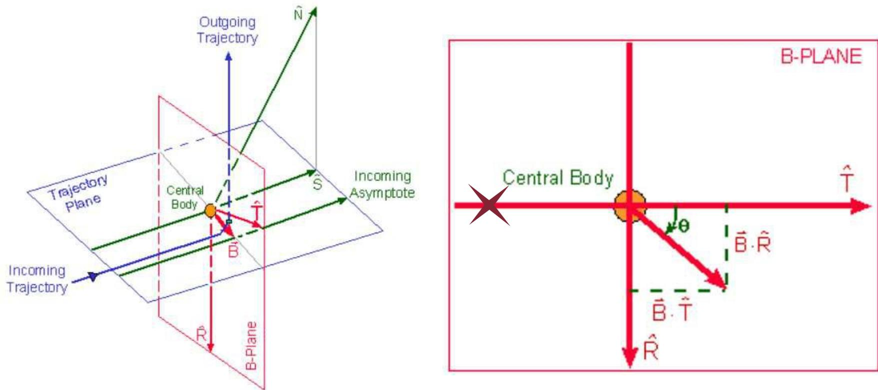
Figure 4. In the Left, B-plane perpendicular to the incoming asymptote of the hyperbola. In the Right, the Vectors R and T lie in the b-plane and are used as axes.
