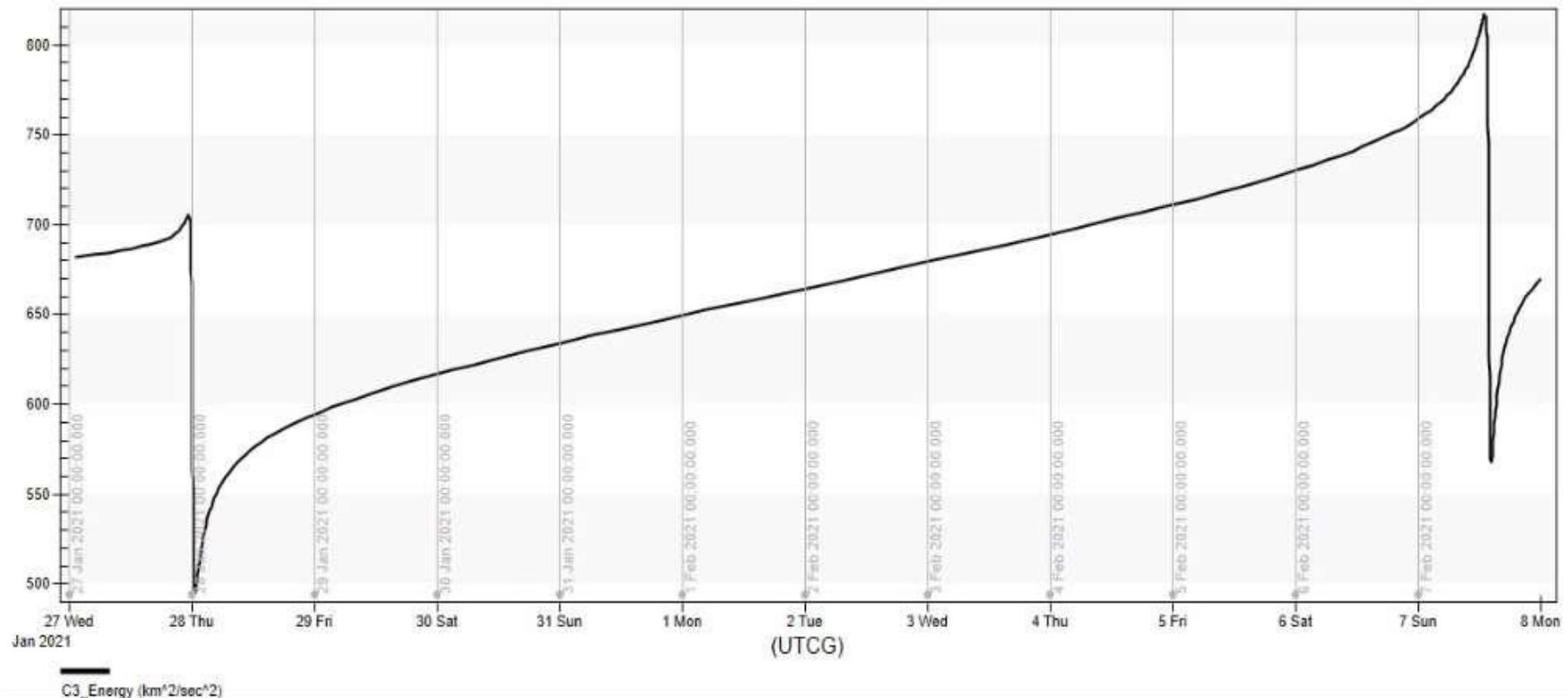
Figure 11. C3 Energy from the Capture Orbit, with 11 days Orbital Period, relative to Mars
