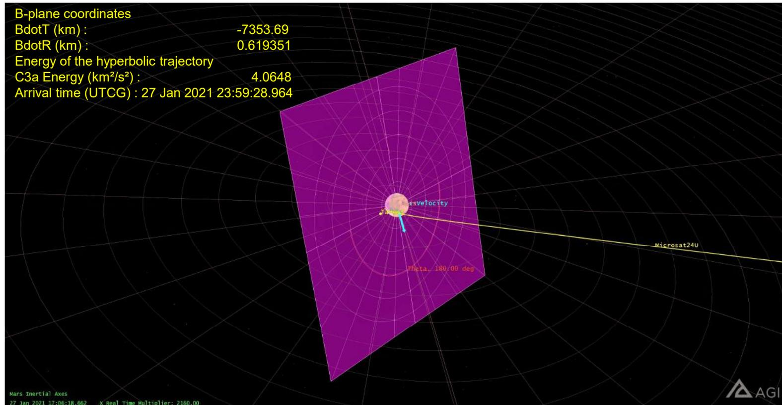
Figure 10. The hyperbolic path values for mars, before entering the capture orbit
