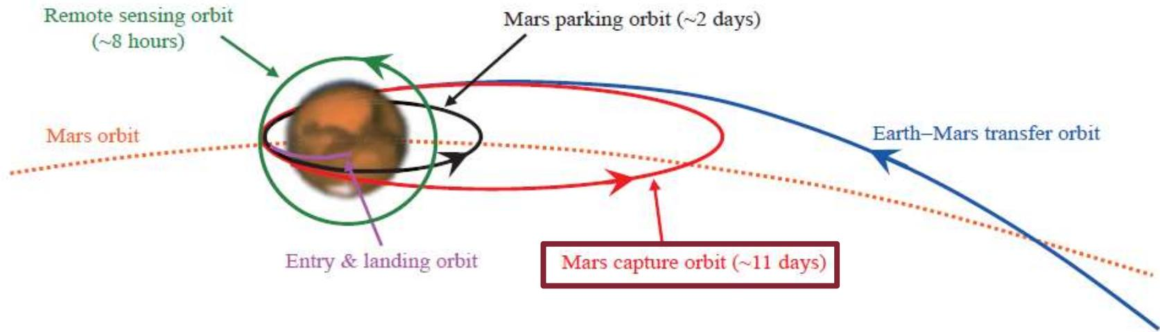
Figure 6. Schematic diagram of the Mars capture, parking, and mission orbits.
