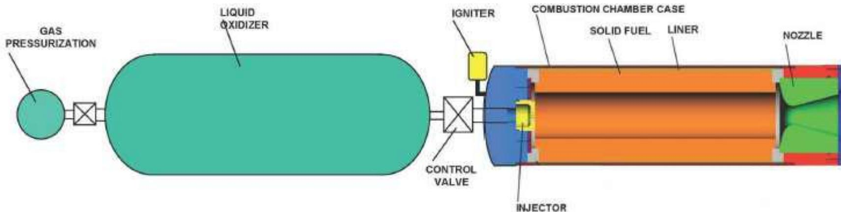
Figure 7. Hybrid rocket engine schematic
