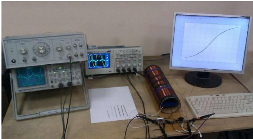
Laboratory facility for the hysteresis damper parameters determination
