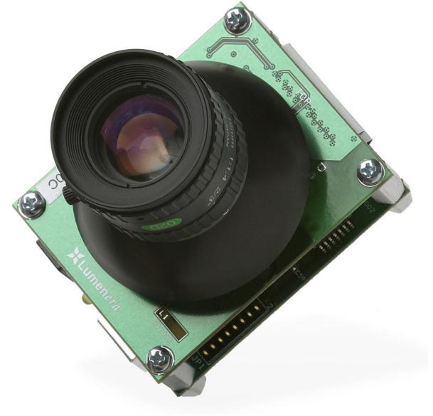
CMOS Sensor and lens
