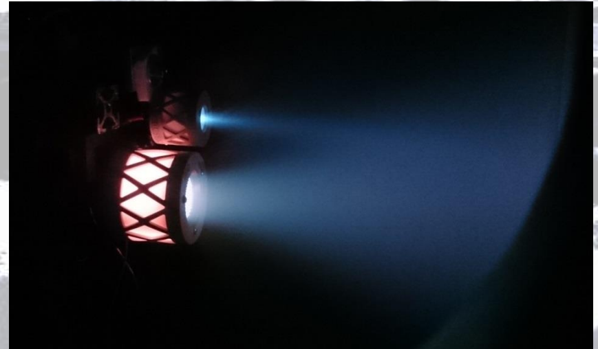
BIT-3 Thruster Firing at the Busek Facilities
