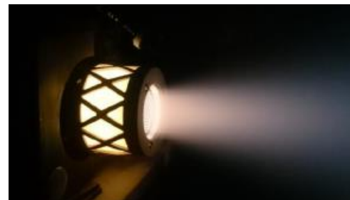
BIT-3 Firing with Iodine propellant at 58W
