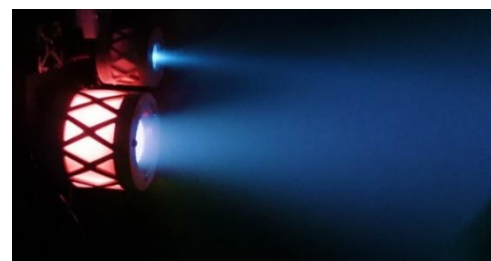
RF cathode operating together with the BIT-3 thruster, both on xenon propellant
