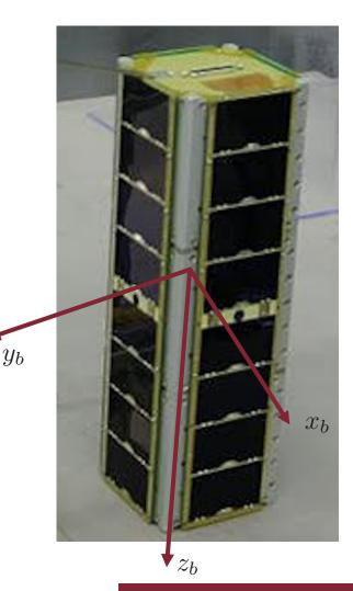
$J_x = J_y = 4.09 \cdot 10^{-2} \text{ kg m}^2$   $J_z = 6.5 \cdot 10^{-3} \text{ kg m}^2$ circular orbit altitude = 629 km  $T_{orbit} = 5832 \text{ sec}$ inclination = 97° RAAN = 68.5°
