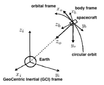
**objective**: stabilize attitude using only magnetorquers so that body frame is aligned with orbital frame (antenna or payload pointing to Earth)
